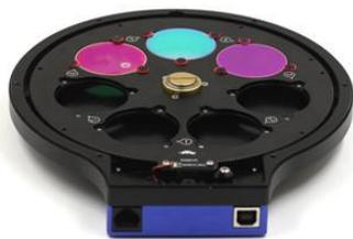
Step 2 Close the top cover: Snap the upper case at the alignment position and secure the eight holes on the edge of the filter wheel with eight flat-head screws. The filter wheel is installed.
