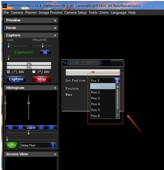
The EZCAP software has a shooting plan function, and setting the corresponding filter wheel hole position in the shooting plan will make shooting easier.
