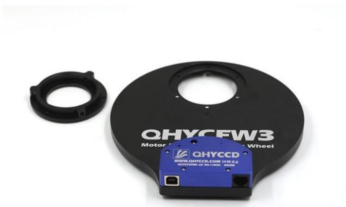
Step 4 Align the new adapter ring with the 6 holes at the bottom of the filter wheel and tighten with screws. (Medium refrigeration COMS series does not need to add adapter ring)
