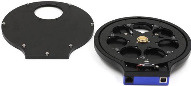
Step 2 Unscrew the upper screw in the middle of the filter disc, loosen the screw of the optocoupler plate, and remove the filter disc.
